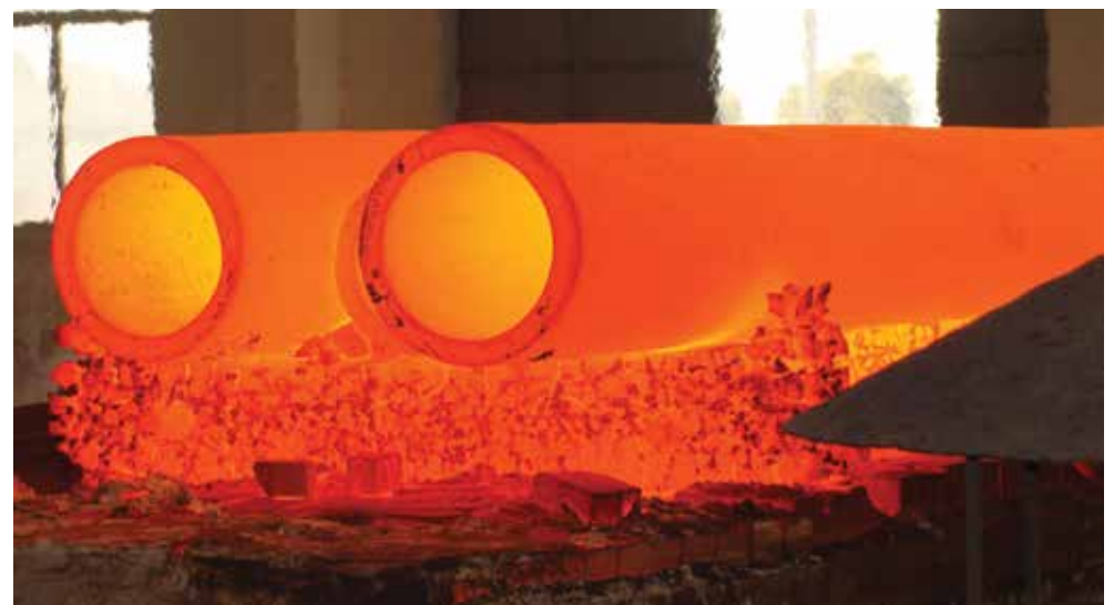
Natural gas tank type heat treatment furnace.
