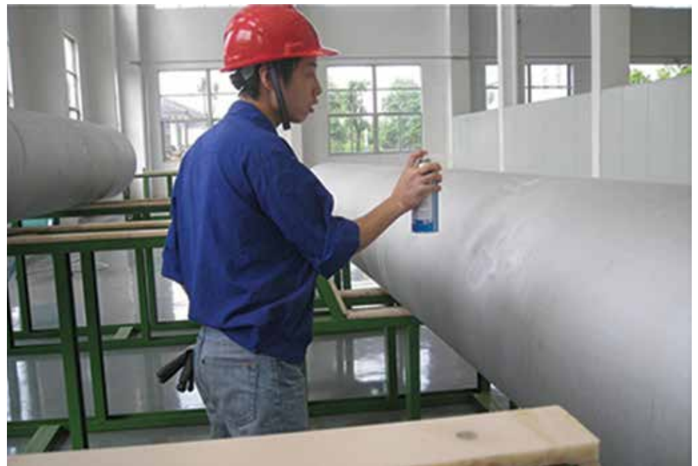
A PT test on a NO8825 large heavy wall seamless pipe.
